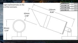
Artemis, Illumicare's adjustable wall mount directional luminaire, is a precision engineered fixture designed for spot, up, and down lighting applications where you need the fixture to be elegant, yet unobtrusive. The contemporary design of the shroud masks the land directs the ight output to eliminate unsightly glare.
