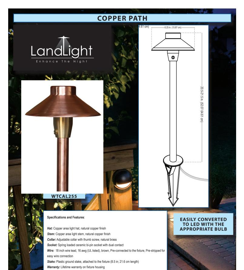
*Certifications:* Complies with the requirements of UL-1838 and CAN/CSA-C22.2 No. 250.7. Identified with the ETL and cETL Listed Mark.
